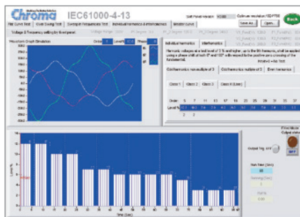
Voltage Harmonic & Interharmonic Test
